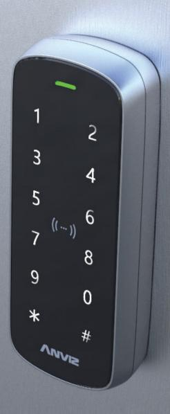
M3 Pro is a metal casing, IP65 water-proof design compact access control device, suitable for outdoor applications. It supports 13.56MHZ mifare card and 125KHZ EM card dual frequency module. The touch backlit keypad, support TCP/IP and RS485 communication convenient for customers to use. The M3 Pro has both built-in relay for direct lock and standard wiegand output, which can be work as standalone access controller and RFID reader.
